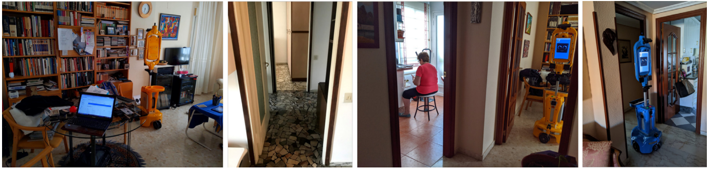
Fig. 4. Pictures of different apartments where the Giraff-X robot was installed. As can be seen, different flooring types, cluttered areas, and narrow doorways are common in these environments, making autonomous navigation a challenging task.
